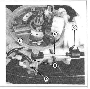
8. Tighten stator plate friction screw (A).
